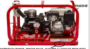
UNDERNEATH ENGINE, REMOVE BOLTS, WASHERS & LOCKNUTS FROM BOTH SIDES, SAVE TO USE FOR STEP 4
