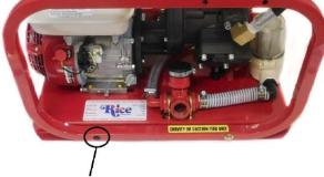
UNDER ENGINE REMOVE BOLTS, WASHERS, & LOCKNUTS FROM BOTH SIDES. SAVE TO USE FOR STEP 4
