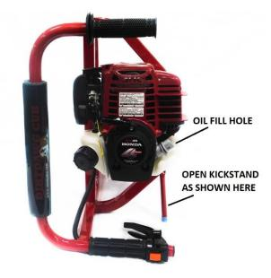
Step 3. Slowly Fill engine with 4-stroke automotive SAE 10W-30 detergent oil. Use supplied bottle of oil which contains 3.4 ounces to avoid overfilling engine.
