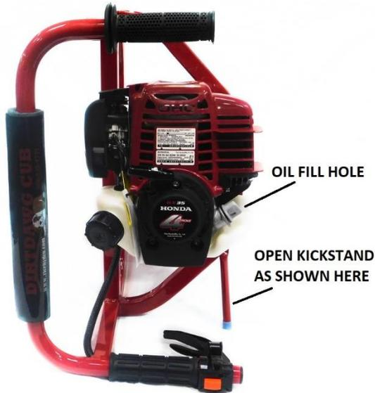
Step 2. To check oil level, use oil filler cap/dipstick to see how much oil is needed.
