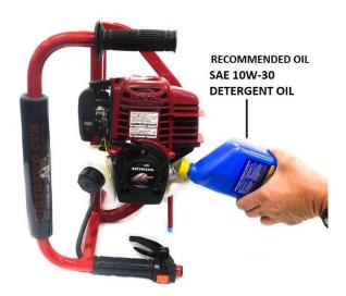
Step 2. To check oil level, use oil filler cap/dipstick to see how much oil is needed. Step 4. Reinstall the oil filler/dipstick securely. If any oil is spilled, make sure to wipe it up.
