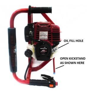
Step 3. Slowly Fill engine with 4-stroke automotive SAE 10W-30 detergent oil. Start with less than 2.7 US ounces and fill to the bottom edge of the oil fill hole as shown on the picture below.
